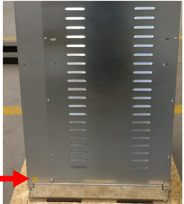
Picture 16 - Screw for the connection of the mass of the storage system to the user's earthing system
