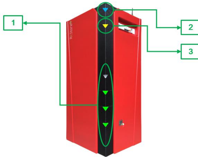
Picture 46 – Status led lights of the storage system
