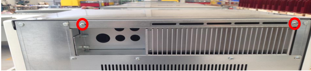
Picture 59 – Replacement of the upper panel in its location
