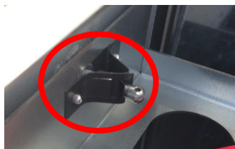
Picture 3 - Removal of the front panel
