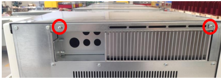
Picture 2 - Removal of the fixing screws of the upper panel
