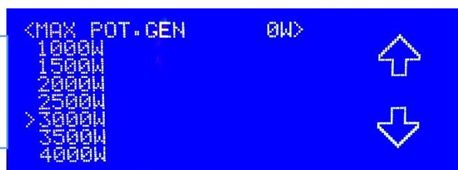
Picture 60 - Gen Diesel: setting up of the parameter “Max Pot.Gen”
