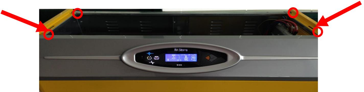
Picture 4 – Removal of lateral panels
