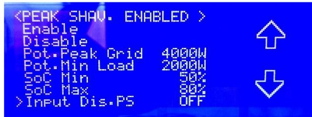
Picture 69 - Peak Shaving: example of setting up of the working parameters; the inhibition entry is not enabled
