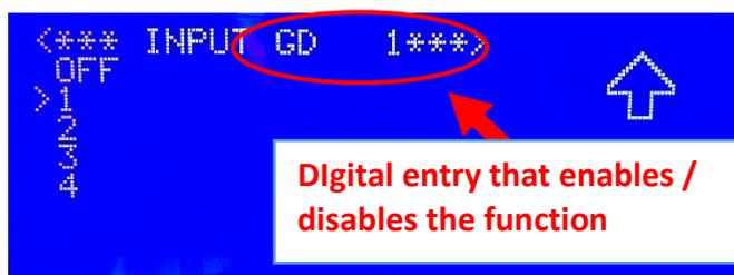
Picture 62 - Gen Diesel: choice of the digital entry available on the control card of the machine that enables/disables the function "GEN DIESEL"
