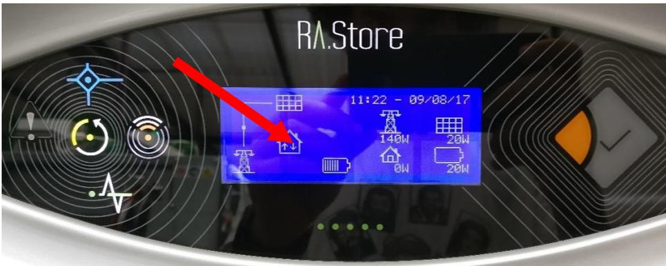
Picture 27 – The double arrows with alternate direction show that the storage system exchanges information with Aton portal
