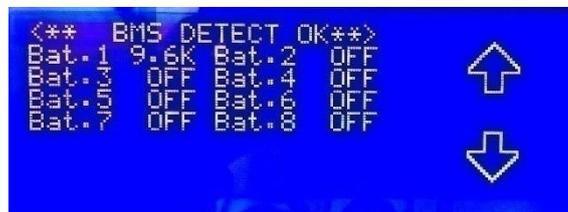
Picture 81 - BMS Detect: procedure finished, 1 identified battery
