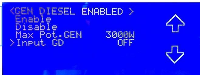
Picture 61 - Gen Diesel: setting up of the parameter "Input GD"
