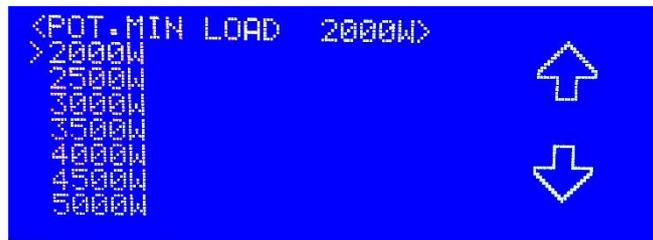
Picture 66 - Peak Shaving: setting up of the parameter Pot. Min Load
