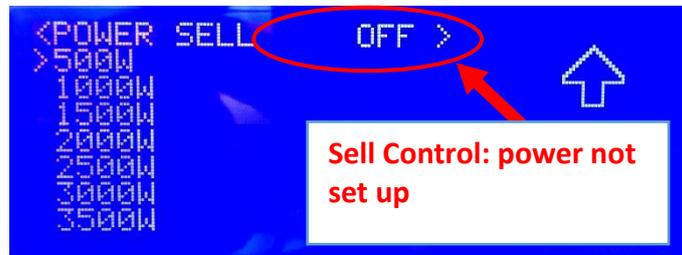
Picture 55 - Sell Control: Screen of setting up “Power Sell”, the value of power given to the grid beyond which it switch over the relay RL2 (OUT2) available on the control card of the machine
