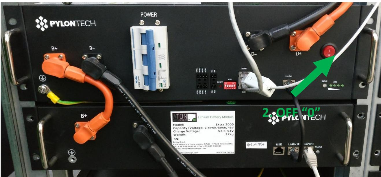
Picture B2 – Red button "0/1" of the batteries in position "0"
