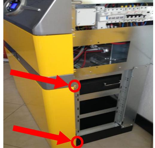
Picture 31 – Screws of the frontal panel
