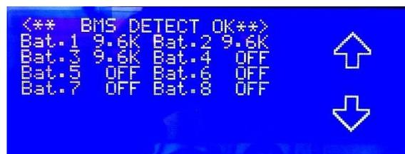
Picture 82 - BMS Detect: procedure finished, 3 identified batteries
