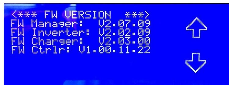
Picture 47 - Info: it visualizes the firmware versions of the components
