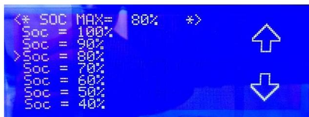
Picture 68 - Peak Shaving: setting up of the parameter SoC Max
