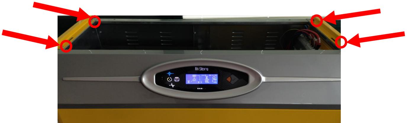
Picture 32 - Screws of the lateral panels
