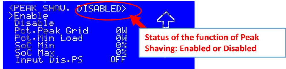
Picture 64 - Peak Shaving: starting screen without parameterization
