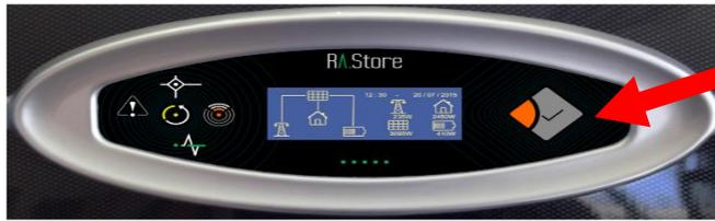
Picture 36 – Access to the setting up menu: press the Enter key
