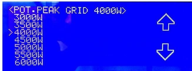
Picture 65 - Peak Shaving: setting up of the parameter Pot. Peak Grid
