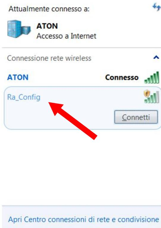
Picture 87 – Connect the PC or smart device to the network Ra\_Config
