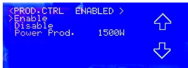
Picture 72 - Production Control: example of setting up of working parameters
