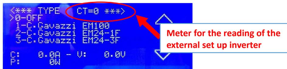
Picture 73 - External Inverter: choice of the meter Carlo Gavazzi
