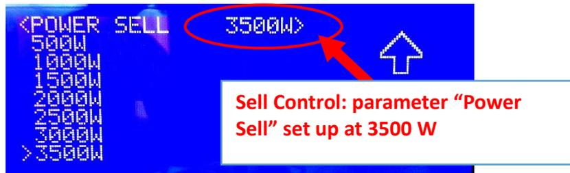
Picture 56 - Sell Control: Screen of setting up “Power Sell”, the value of power given to the grid beyond which it switch over the relay RL2 (OUT2) available on the control card of the machine; example of setting up at 3500 W
