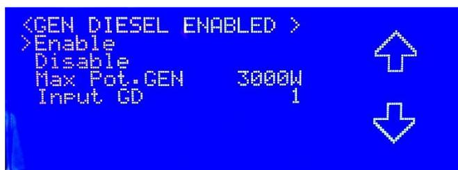
Picture 63 - Gen Diesel: final screen after having set up all the parameters regarding the functioning
