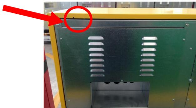
Picture 10 – Slot for the antenna cable
